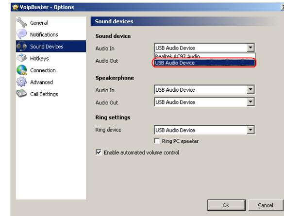
Set “Sound device”, “Speakerphone” and “Ring settings” to “USB Audio Device”.
