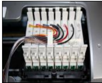
Insert our no-sponge cartridge into printer carefully
