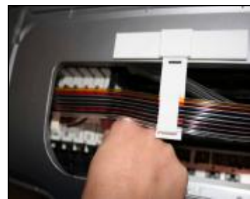
Make sure the lengh of tubeline is enough to reach the far left and right
