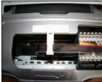
Insert the tubeline into the Support arm
