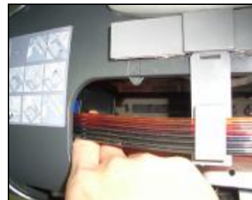
Make sure the lengh of tubline is enough to reach the far left and right
