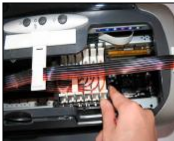
Adjust the tubeline,remove the Cartridge-car back and forth
