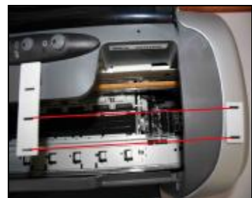
Attached the clamp on your printer and let it parallel with printer
