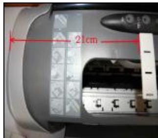
Fix the arm on the 21cm right far from you printer
