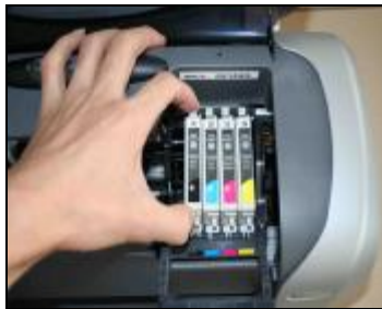
Remove original cartridge
