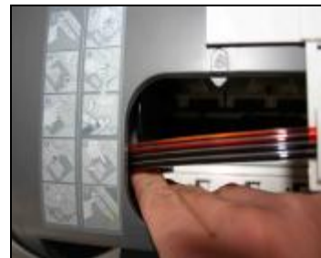
Make sure the lengh of tubline is enough to reach the far left and right
