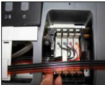
Make sure tubeline will not meet printer when printing
