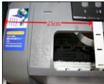
Fix the arm on the 25cm right far from you printer
