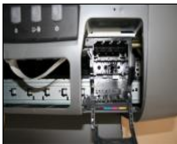
Remove original cartridge
