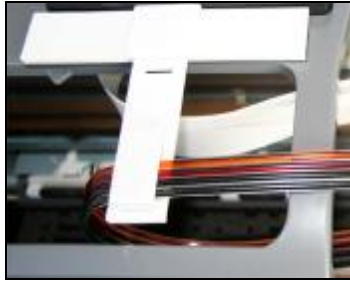
Insert tubeline through the arm
