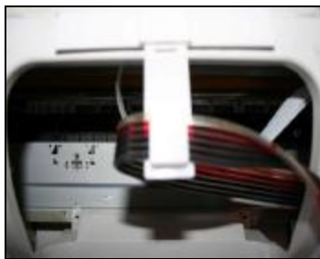
Insert tubeline through the arm
