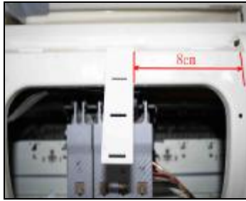
Fix the arm on the 8cm right far from you printer
