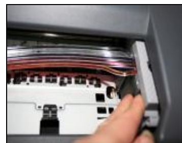
Make sure the lenth of tubline is enough to reach the far left and right
