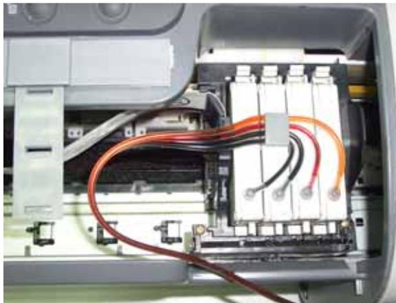
9. Put the Tube into the Support Arm and Small Tube clamp as the below picture shown.
