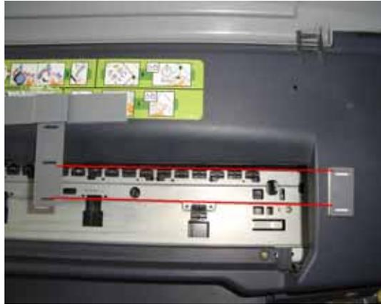
8. Insert the cartridge into the cartridge carriage after finishing ink-filling; Make sure the cartridge is down all the way and they are making contact with the fingers that read chips; Then close the CIS Cover.
