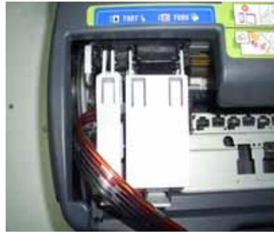
9. Put the Tube into the Support Arm and Small Tube clamp as the below picture shown.
