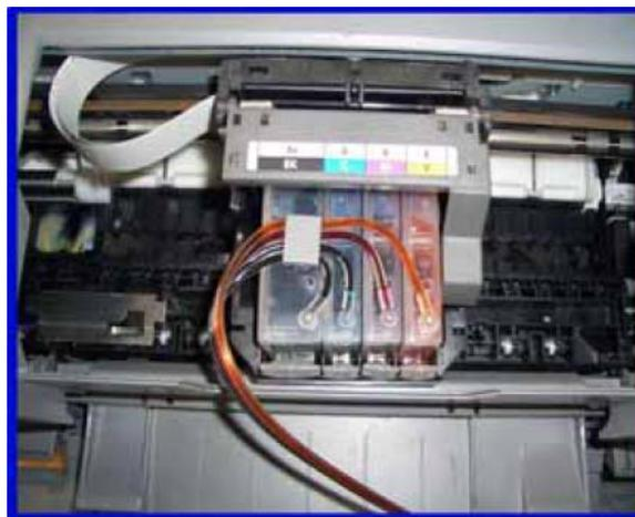
7. Put the Tube into the Support Arm and Small Tube clamp as the below picture shown.
