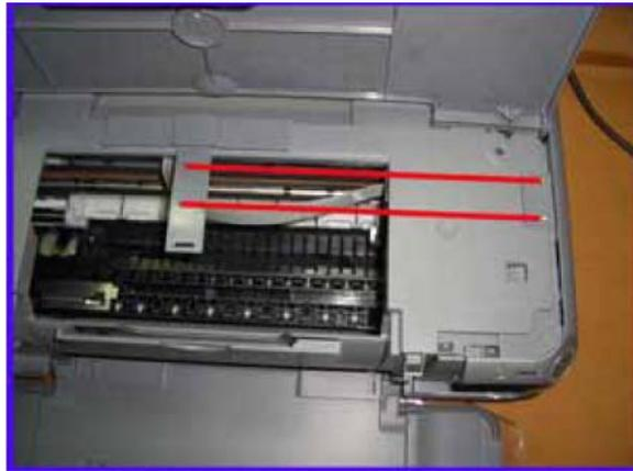
6. Insert the cartridge into the cartridge carriage; Make sure the cartridge is down all the way and they are making contact with the printer;
